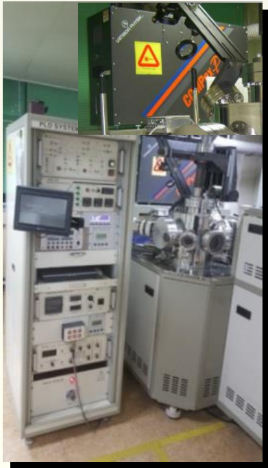
PLD system (Pulsed Laser Deposition)
