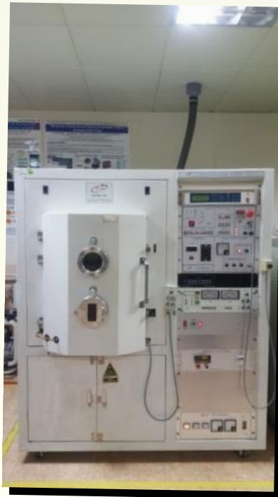
E-Beam evaporator
