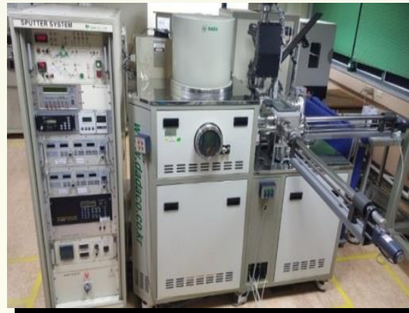
Magnetron sputter system (DC/RF)
